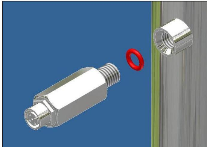
Carry out the hydraulic test, verifying that the o-rings are watertight and that there're not water leaks outside the sleeve bolts or inside the quartz sleeves.
