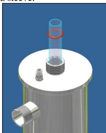
Screw again the sleeve bolts and insert the lamp holder spring into the sleeve:
