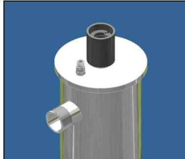
Insert the quartz sleeves carefully centring the spring at the bottom plate of the UV chamber:
