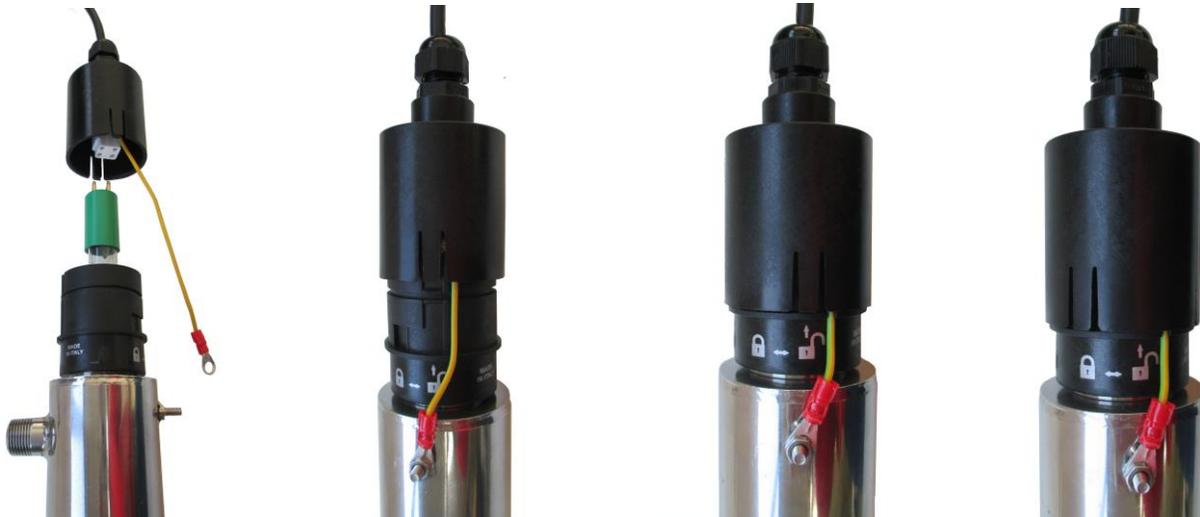
Finally connect the power cable to the socket.
