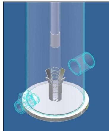
Insert the o-ring Ø 23x4 into the quartz sleeve:
